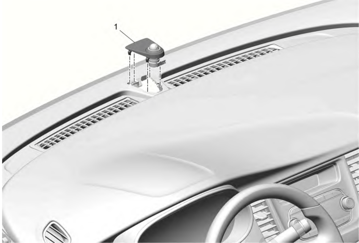
Fig. 38: Sun Load Temperature Sensor Bezel Courtesy of GENERAL MOTORS COMPANY
